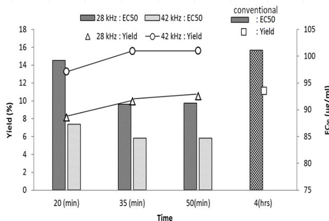
Figure 2. Effect of time on the yield and  $EC_{50}$  values in the UAE methods and compared to the conventional method. Both experiments were conducted at constant temperature of 45°C (Hadiyanto *et al.*, 2016).
