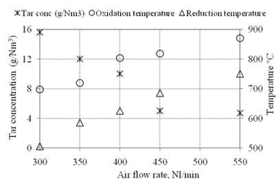
Figure 5. Quantity of tar, oxidation temperature and reduction temperature with air flow rates.
