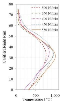
Figure 4. Temperature profiles for various air flow rates.
