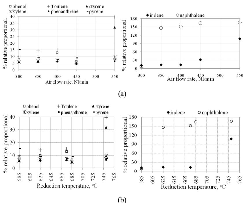
Figure 8. Evolution of tar compounds (a) with air flow rate and (b) with reduction temperature.
