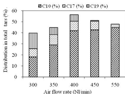
Figure 7. Distribution of C<sub>10</sub>, C<sub>17</sub> and C<sub>19</sub> in the GC detectable tars.
