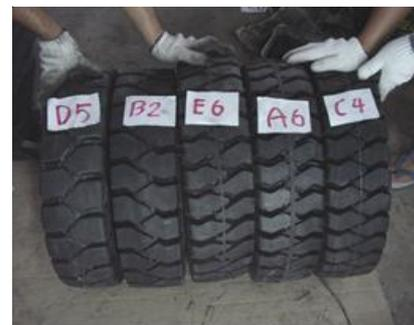
Figure 2. Tire specimens size 6.00-9 of five different brands.
