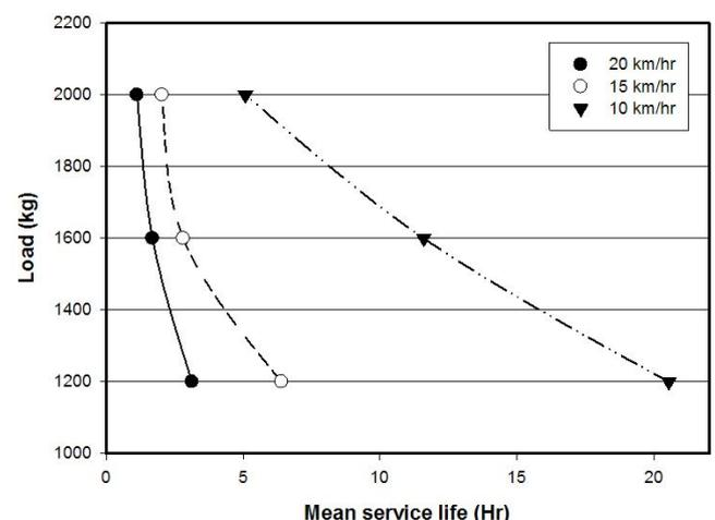
Figure 3. Mean service life of solid tires size 6.00-9 at various test speeds.
