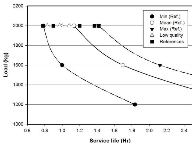
Figure 4. Service life of solid tires size 6.00-9 at test speed of 20 km/hr.
