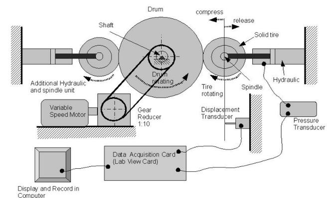
Figure 1. Drum-like testing machine.
