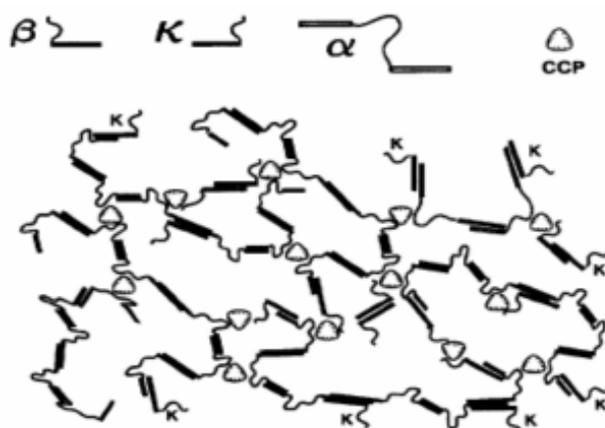
Figure 13. The dual bonding model of casein micelle structure, with  $\alpha$ -,  $\beta$ -,  $\kappa$ -casein portrayed as indicated. Bonding appears between the hydrophobic regions, shown as rectangular bars, and by linkage of hydrophilic regions containing phosphoserine clusters to colloidal calciumphosphate clusters. Molecules of  $\kappa$ -casein (K) limit further growth of the structure. (Source: Horne, 1998)
